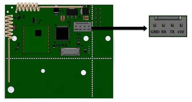
uartBridge via UART interface provides a data flow rate at 57,600 bps
